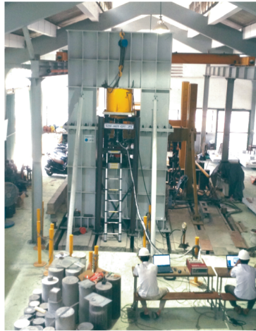
Photo 3 Compression loading test setup
